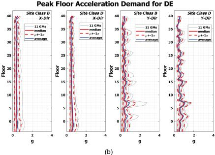
Figure 3-6 Earthquake demands from non-linear response history analysis of the steel buckling-restrained braced frame building under the design earthquake: (a) transient story drifts and (b) floor accelerations.
