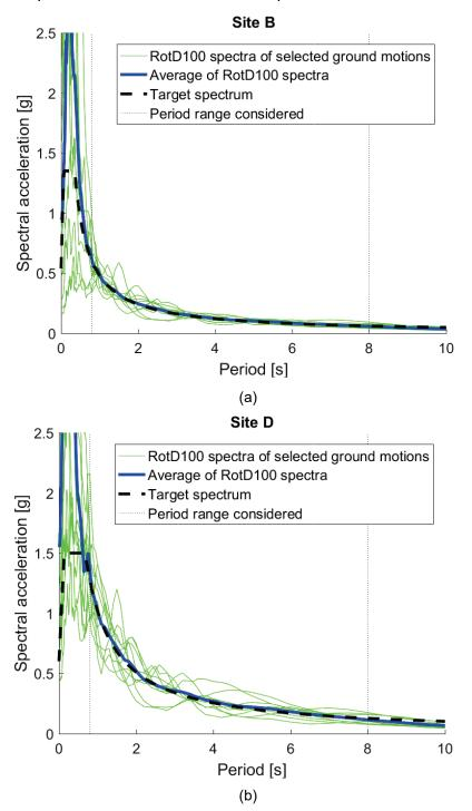
Figure 3-4 Maximum Considered Earthquake (MCE) target spectrum superimposed with the average and individual ground motion spectra for (a) Site Class B; and (b) Site Class D locations.
