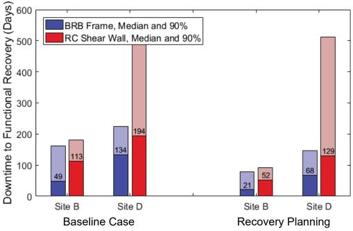
Figure 3-10 Summary of median and 90th percentile functional recovery time considering the baseline case and recovery planning under DE shaking.
