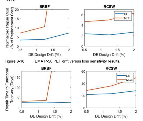
Figure 3-19 FEMA P-58 PET drift versus repair time sensitivity results.
