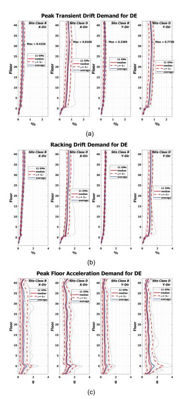
Figure 3-5 Earthquake demands from non-linear response history analysis of the reinforced concrete shear wall residential building under the design earthquake: (a) transient story drifts; (b) racking story drifts; and (c) floor accelerations.
