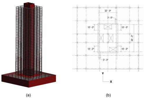
Figure 3-1 Reinforced concrete shear wall residential building (a) isometric view and (b) superstructure plan view. Adapted from Almufti et al. (2018).
