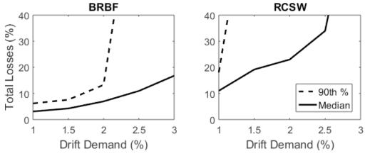
Figure 3-13 Mean story drift demand versus repair cost losses.
