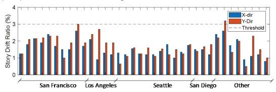
Figure 3-16 Mean MCE-level story drift demands from recently completed tall buildings designed using performance-based methods.
