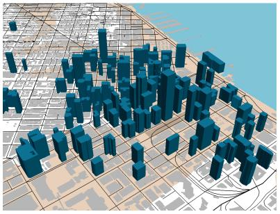
Figure 1-2 Spatial distribution of San Francisco's tall building inventory. Footprints of buildings not included in the inventory are shown for reference. Beige denotes liquefaction zone (per DataSF).
