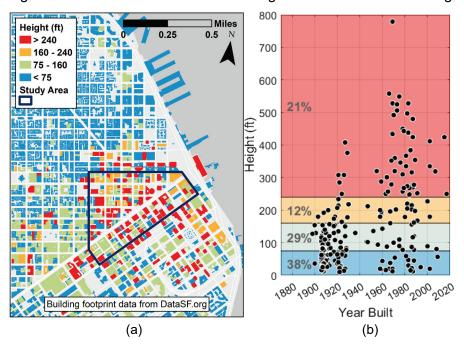
Figure 1-7 Map showing 243 buildings in a 31-block downtown San Francisco study area: (a) the study area, focused on the blocks with the highest concentrations of tall buildings; and (b) the height and dates of buildings in the study area, with the percent in each height category.
