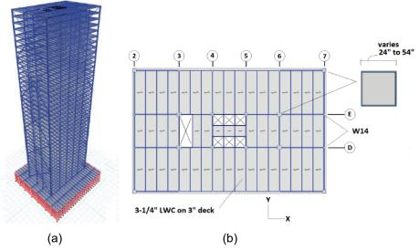
Figure 3-2 Buckling-restrained braced frame office building (a) isometric view and (b) superstructure plan view.
