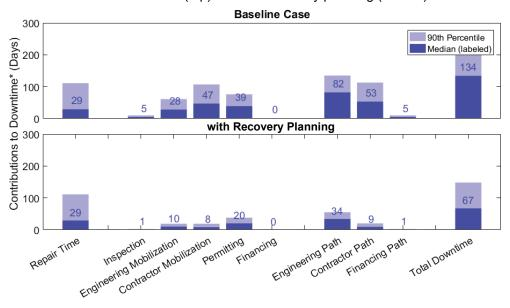
Figure 3-12 Steel BRB functional recovery time deaggregation at Site Class D under DE: baseline (top) and with recovery planning (bottom).
