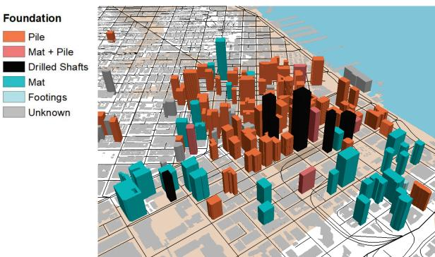
Figure 2-1 Map showing foundation types of tall buildings superimposed where beige shading identifies regions that are susceptible to soil liquefaction during strong earthquakes (soil information from https://datasf.org/).
