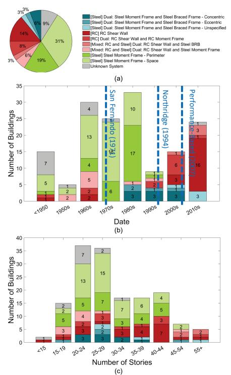
Figure 1-3 Figure showing 156 San Francisco buildings tall than 240 ft by: (a) percentage of buildings by SFRS type, (b) breakdown of SFRS by decade, and (c) distribution of SFRS by number of stories.
