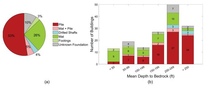
Figure 1-6 Figure showing: (a) percentage of buildings by foundation type, and (b) breakdown of foundation types by depth to bedrock.
