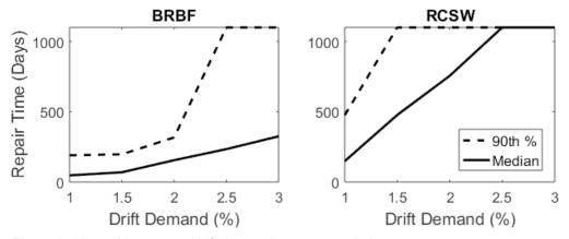
Figure 3-14 Mean story drift demand versus repair times.
