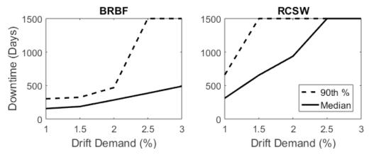
Figure 3-15 Mean story drift demand versus functional recovery times.
