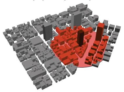
Figure 5-2 Illustration of a tall building cordon around a hypothetical 520-ft tall building with a cordon radius equal to 1.5 times the building height.
