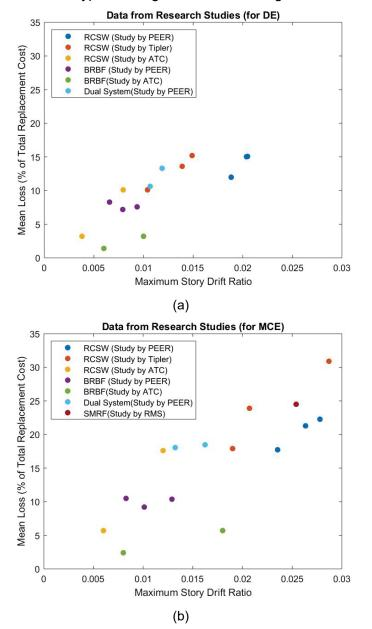
Figure 3-17 Loss versus drift data for different structural systems at (a) DE and (b) MCE ground motion intensities.
