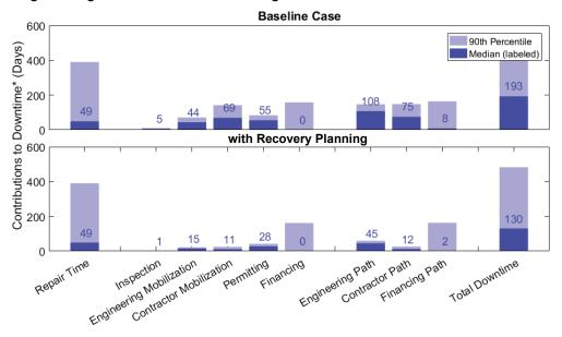
Figure 3-11 RCSW functional recovery time deaggregation at Site Class D under DE: baseline (top) and with recovery planning (bottom).
