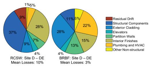
Figure 3-9 Contribution of different building components to overall loss at DE for Site Class D.
