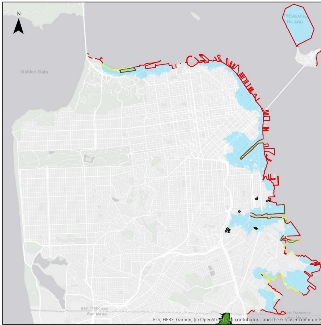
FIGURE A-65: SHORELINE PROTECTION AND FLOOD HAZARD (100 YEAR STORM + 66" SEA LEVEL RISE)
