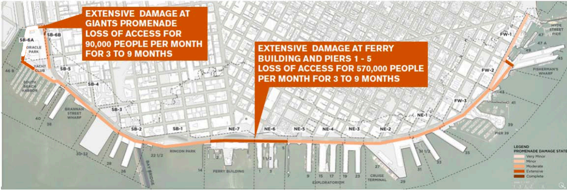
Figure 2-4. Promenade Damage States for 225-year Seismic Event
