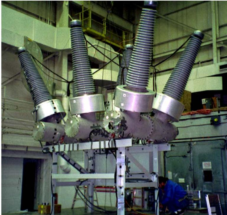
Seismic Tests on Replacement Breakers
