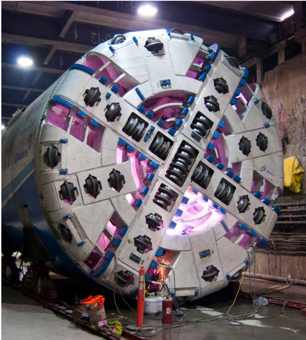
Central Subway Boring Machine
